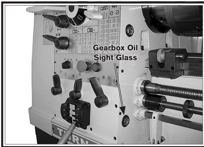
Figure 102. Location of quick-change gearbox oil sight glass.
